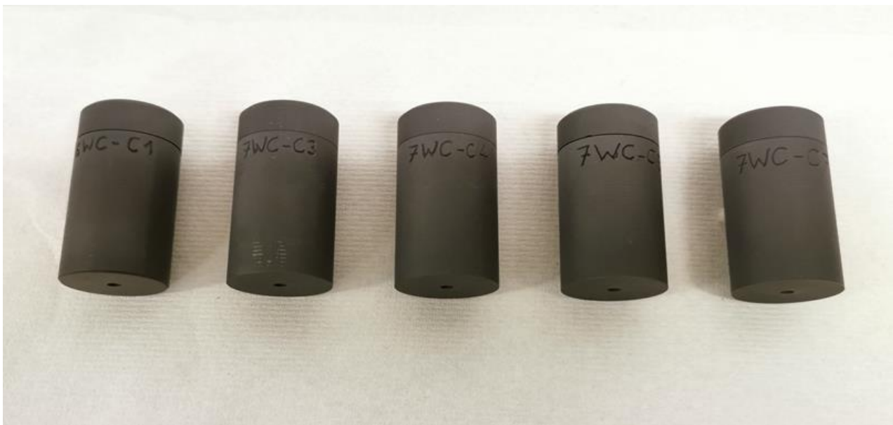
Figure 2: set of 5 WC-C cells based on the hybrid design (sleeve and CC sheets) constructed at LNE-Cnam using the piston method
