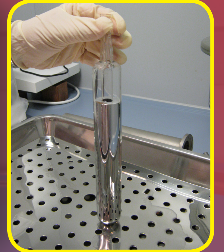
Typical mercury cell
